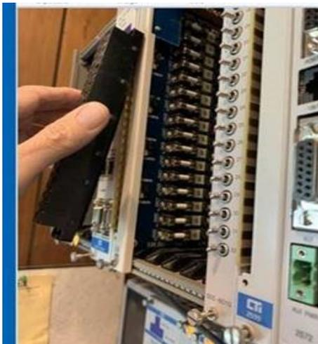
Step 2: Once the connector is inserted at the top roll the connector down while pushing the connector in to completely insert it on the board.
