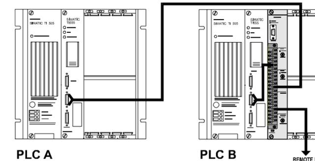
The remote I/O port of PLC A and PLC B are both connected to the appropriate terminals on the RPM. The cable from the remote I/O is connected to the module. Three sets of nine additional terminals are provided for switching the connections between operator interface devices and the PLC communication ports. These connections are not shown in the figure above. See wiring diagram on back page for details.
