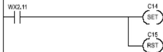
C14 is used as a flag which indicates that the command cycle was started. The cycle starts when Command Busy (WX2.11) comes on. C15 is reset at the beginning of a command cycle.
