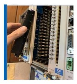
Step 3: Once you have rolled the connector all the way down and fully inserted onto the PCB you can finish the installation by screwing the Thumb Screws down. Do not overtighten.
