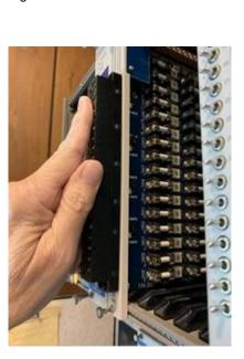
Step 2: Once the connector is inserted at the top roll the connector down while pushing the connector in to completely insert it on the board.
