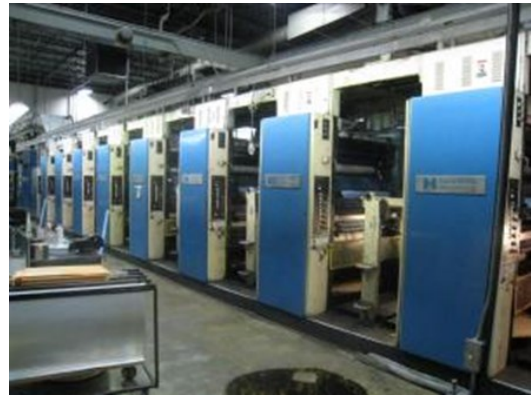
Figure 3: M1000B Printing Press
