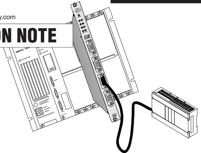
The CTI 2573-TCM2 Serial Interface Adapter allows the Simatic® 505 data using the Modbus Protocol.
