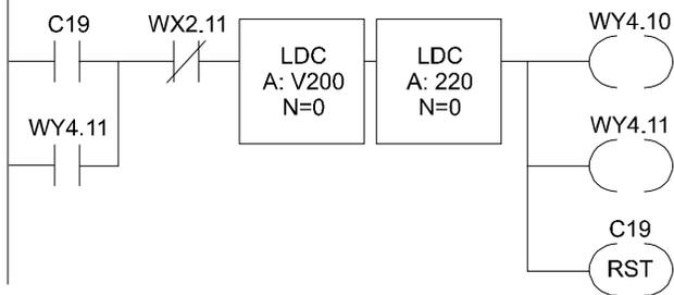
This rung is the command trigger for coupled mode. The Command Error words in both command blocks are cleared when a new command cycle is initiated.
