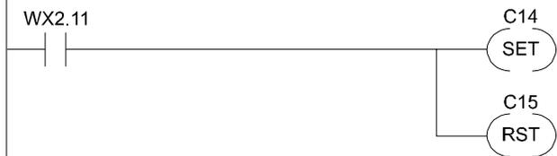
C14 is used as a flag which indicates that the command cycle was started. The cycle starts when Command Busy (WX2.11) comes on. C15 is reset at the beginning of a command cycle.
