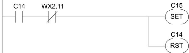
Once the command cycle is started (C14 is on), when command busy goes off, the command cycle is complete. The Cycle Complete flag (C15) is set and C14 is reset.
