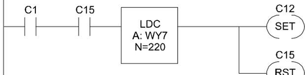
If C1 is on, then WY7 contains the address of the Create Connection Command Block. When C15 is on, the module has completed a command cycle. When both events are true, you have successfully created a connection and are ready for the Send Query Command. This rung load WY7 with the address of this Command Block (V220), sets C12 to indicate this and reset the Cycle Complete flag (C15).
