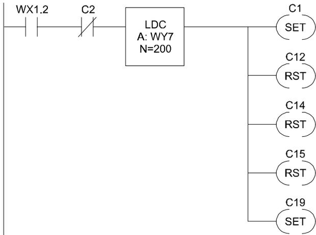
This rung selects the Create Connection Command Block by loading the V memory address of 200 in WY7. The 2573-MOD will turn the WX1.2 (SER CFG) bit on when the module is reset; it will remain on until all ports have been configured (either by DIP switch or by a Create Connection). Thus this rung is executed when WX1.2 first goes high.
