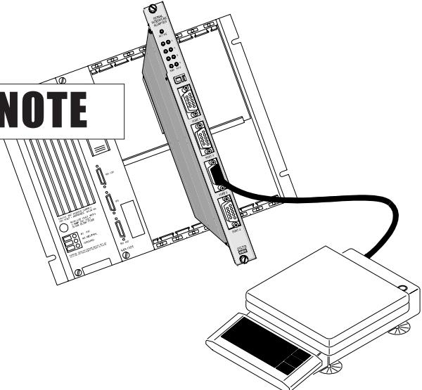
The CTI 2573-TCM2 Serial Interface Adapter is used to include the Mettler/Toledo PG5001 scale in a Simatic® 505 PLC system.
