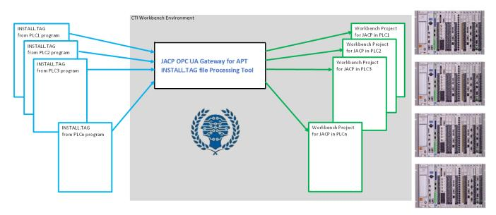
This hardware and software combination allows you to program/online-update the JACP(s) in a matter of seconds to function as an OPC UA server that seamlessly interfaces with the CTI 2500 Series Cx00 (or Legacy Siemens 505) Processor running your APT or FTS programs via the CTI Enhanced Data Cache.
