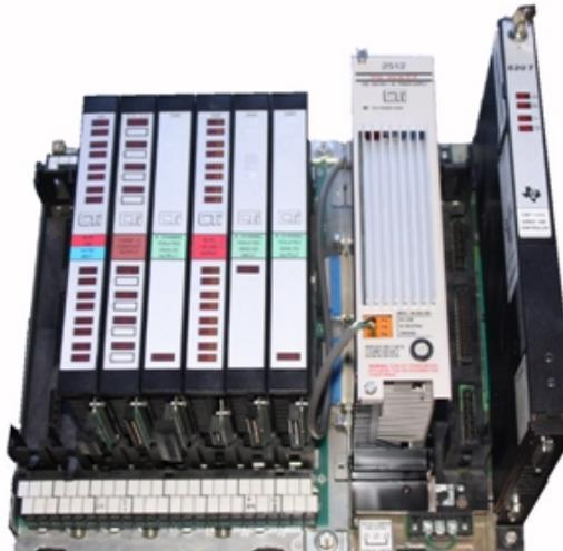
Although the IOCC/DBC architecture was not a part of the 560 system (predated it), CTI also has a product to replace the very old “oil pan” format of the 520/530 PLC. This 2500-R4500 (available August 2009) can also replace the smaller Distributed Base Controllers (DBC).
