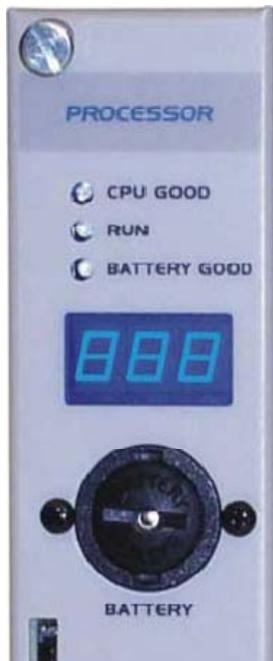
The IP address is displayed on the Multi Segment Display on the Front Panel. The 4 octets of the IP address are cyclically displayed one after the other, separated by a dot after the lowest octet.
