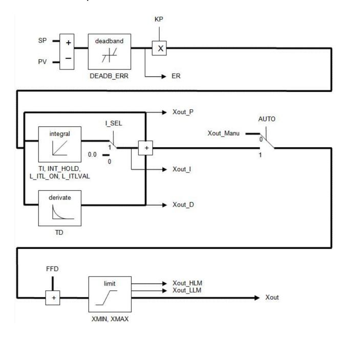
The PID instruction in Workbench is supported in Ladder Diagram (LD), Function Block Diagram (FBD), and Structured Text (ST) programming languages.
