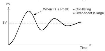
The I control is not used by itself. It is used with P (PI control) or P and D (PID control).
