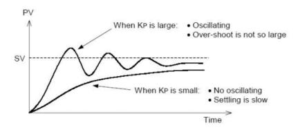
With just P control, an offset (residual error) will remain. Therefore, P control is used with I control (PI
