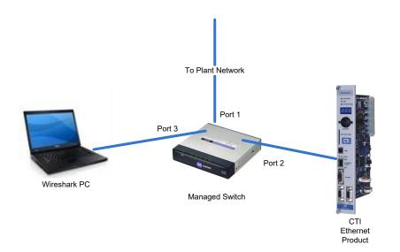
Figure 1. Network Capture Setup
